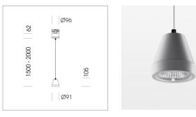
Suspended luminaire with LED, rated life of the LED L80/B10 > 50000 h, colour rendering index CRI > 80, chromaticity tolerance 3 SDCM (initial), rotation-symmetrical reflector with circular light distribution pattern, reflector pure aluminium 99,99% in MIRO-Silver®,segmented and faceted, 3D lens silicon to reduce the proportion of scattered light, luminaire head die-cast aluminium, powder-coated, stratosilver
