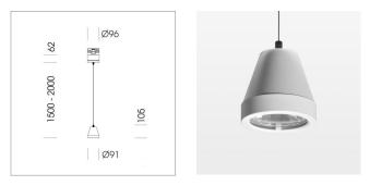
Suspended luminaire with LED, rated life of the LED L80/B10 > 50000 h, colour rendering index CRI > 90, chromaticity tolerance 3 SDCM (initial), rotation-symmetrical reflector with circular light distribution pattern, reflector pure aluminium 99,99% in MIRO-Silver®,segmented and faceted, 3D lens silicon to reduce the proportion of scattered light, luminaire head die-cast aluminium, powder-coated, stratowhite
