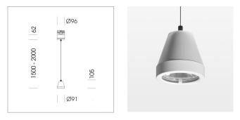
Suspended luminaire with LED, rated life of the LED L80/B10 > 50000 h, colour rendering index CRI > 96, chromaticity tolerance 2 SDCM (initial), rotation-symmetrical reflector with circular light distribution pattern, reflector pure aluminium 99,99% in MIRO-Silver®,segmented and faceted, 3D lens silicon to reduce the proportion of scattered light, luminaire head die-cast aluminium, powder-coated, stratowhite
