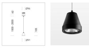
Suspended luminaire with LED, rated life of the LED L80/B10 > 50000 h, colour rendering index CRI > 90, chromaticity tolerance 2 SDCM (initial), rotation-symmetrical reflector with circular light distribution pattern, reflector pure aluminium 99,99% in MIRO-Silver®,segmented and faceted, 3D lens silicon to reduce the proportion of scattered light, luminaire head die-cast aluminium, powder-coated, stratoblack
