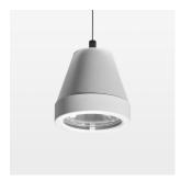
Suspended luminaire with LED, rated life of the LED L80/B10 > 50000 h, colour rendering index CRI > 90, chromaticity tolerance 2 SDCM (initial), rotation-symmetrical reflector with circular light distribution pattern, reflector pure aluminium 99,99% in MIRO-Silver®, segmented and faceted, 3D lens silicon to reduce the proportion of scattered light, luminaire head die-cast aluminium, powder-coated, stratowhite
