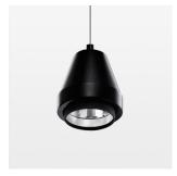
Suspended luminaire with LED, rated life of the LED L80/B10 > 50000 h, colour rendering index CRI > 80, chromaticity tolerance 2 SDCM (initial), reflector with circular light distribution pattern, reflector pure aluminium 99,99% in MIRO-Silver®, segmented and faceted, 3D lens silicon to reduce the proportion of scattered light, luminaire head die-cast aluminium, powder-coated, stratoblack
