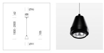
Suspended luminaire with LED, rated life of the LED L80/B10 > 50000 h, colour rendering index CRI > 96, chromaticity tolerance 3 SDCM (initial), reflector with circular light distribution pattern, reflector pure aluminium 99,99% in MIRO-Silver®,segmented and faceted, 3D lens silicon to reduce the proportion of scattered light, luminaire head die-cast aluminium, powdercoated, stratoblack
