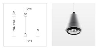
Suspended luminaire with LED, rated life of the LED L80/B10 > 50000 h, colour rendering index CRI > 90, chromaticity tolerance 2 SDCM (initial), reflector with circular light distribution pattern, reflector pure aluminium 99,99% in MIRO-Silver®,segmented and faceted, 3D lens silicon to reduce the proportion of scattered light, luminaire head die-cast aluminium, powdercoated, stratowhite
