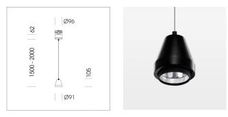
Suspended luminaire with LED, rated life of the LED L80/B10 > 50000 h, colour rendering index CRI > 80, chromaticity tolerance 2 SDCM (initial), reflector with circular light distribution pattern, reflector pure aluminium 99,99% in MIRO-Silver®,segmented and faceted, 3D lens silicon to reduce the proportion of scattered light, luminaire head die-cast aluminium, powdercoated, stratoblack
