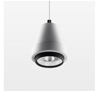
Suspended luminaire with LED, rated life of the LED L80/B10 > 50000 h, colour rendering index CRI > 80, chromaticity tolerance 2 SDCM (initial), reflector with circular light distribution pattern, reflector pure aluminium 99,99% in MIRO-Silver®, segmented and faceted, 3D lens silicon to reduce the proportion of scattered light, luminaire head die-cast aluminium, powder-coated, stratowhite
