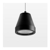
Suspended luminaire with LED, rated life of the LED L80/B10 > 50000 h, chromaticity tolerance 2 SDCM (initial), reflector with circular light distribution pattern, reflector pure aluminium 99,99% in MIRO-Silver®,segmented and faceted, 3D lens silicon to reduce the proportion of scattered light, luminaire head die-cast aluminium, powder-coated, stratoblack
