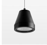
Suspended luminaire with LED, rated life of the LED L80/B10 > 50000 h, colour rendering index CRI > 90, chromaticity tolerance 2 SDCM (initial), reflector with circular light distribution pattern, reflector pure aluminium 99,99% in MIRO-Silver®,segmented and faceted, luminaire head die-cast aluminium, powder-coated, stratoblack
