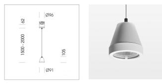
Suspended luminaire with LED, rated life of the LED L80/B10 > 50000 h, colour rendering index CRI > 90, chromaticity tolerance 2 SDCM (initial), reflector with circular light distribution pattern, reflector pure aluminium 99,99% in MIRO-Silver®,segmented and faceted, luminaire head die-cast aluminium, powder-coated, stratowhite
