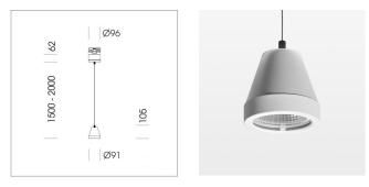
Suspended luminaire with LED, rated life of the LED L80/B10 > 50000 h, colour rendering index CRI > 80, chromaticity tolerance 2 SDCM (initial), reflector with circular light distribution pattern, reflector pure aluminium 99,99% in MIRO-Silver®,segmented and faceted, luminaire head die-cast aluminium, powder-coated, stratowhite
