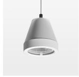
Suspended luminaire with LED, rated life of the LED L80/B10 > 50000 h, chromaticity tolerance 2 SDCM (initial), reflector with circular light distribution pattern, reflector pure aluminium 99,99% in MIRO-Silver®,segmented and faceted, luminaire head die-cast aluminium, powder-coated, stratowhite
