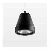
Suspended luminaire with LED, rated life of the LED L80/B10 > 50000 h, colour rendering index CRI > 90, chromaticity tolerance 3 SDCM (initial), rotation-symmetrical reflector with circular light distribution pattern, reflector pure aluminium 99,99% in MIRO-Silver®, segmented and faceted, 3D lens silicon to reduce the proportion of scattered light, luminaire head die-cast aluminium, powder-coated, stratoblack
