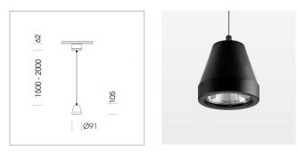
Suspended luminaire with LED, rated life of the LED L80/B10 > 50000 h, colour rendering index CRI > 95, chromaticity tolerance 2 SDCM (initial), rotation-symmetrical reflector with circular light distribution pattern, reflector pure aluminium 99,99% in MIRO-Silver®,segmented and faceted, 3D lens silicon to reduce the proportion of scattered light, luminaire head die-cast aluminium, powder-coated, stratoblack
