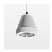
Suspended luminaire with LED, rated life of the LED L80/B10 > 50000 h, colour rendering index CRI > 90, chromaticity tolerance 3 SDCM (initial), rotation-symmetrical reflector with circular light distribution pattern, reflector pure aluminium 99,99% in MIRO-Silver®, segmented and faceted, 3D lens silicon to reduce the proportion of scattered light, luminaire head die-cast aluminium, powder-coated, stratowhite
