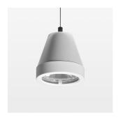
Suspended luminaire with LED, rated life of the LED L80/B10 > 50000 h, colour rendering index CRI > 96, chromaticity tolerance 2 SDCM (initial), rotation-symmetrical reflector with circular light distribution pattern, reflector pure aluminium 99,99% in MIRO-Silver®, segmented and faceted, 3D lens silicon to reduce the proportion of scattered light, luminaire head die-cast aluminium, powder-coated, stratowhite
