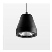
Suspended luminaire with LED, rated life of the LED L80/B10 > 50000 h, colour rendering index CRI > 90, chromaticity tolerance 2 SDCM (initial), rotation-symmetrical reflector with circular light distribution pattern, reflector pure aluminium 99,99% in MIRO-Silver®, segmented and faceted, 3D lens silicon to reduce the proportion of scattered light, luminaire head die-cast aluminium, powder-coated, stratoblack
