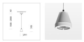
Suspended luminaire with LED, rated life of the LED L80/B10 > 50000 h, colour rendering index CRI > 90, chromaticity tolerance 2 SDCM (initial), rotation-symmetrical reflector with circular light distribution pattern, reflector pure aluminium 99,99% in MIRO-Silver®,segmented and faceted, 3D lens silicon to reduce the proportion of scattered light, luminaire head die-cast aluminium, powder-coated, stratowhite
