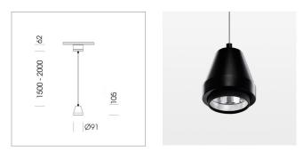
Suspended luminaire with LED, rated life of the LED L80/B10 > 50000 h, colour rendering index CRI > 80, chromaticity tolerance 2 SDCM (initial), reflector with circular light distribution pattern, reflector pure aluminium 99,99% in MIRO-Silver®,segmented and faceted, 3D lens silicon to reduce the proportion of scattered light, luminaire head die-cast aluminium, powdercoated, stratoblack
