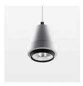
Suspended luminaire with LED, rated life of the LED L80/B10 > 50000 h, colour rendering index CRI > 80, chromaticity tolerance 2 SDCM (initial), reflector with circular light distribution pattern, reflector pure aluminium 99,99% in MIRO-Silver®, segmented and faceted, 3D lens silicon to reduce the proportion of scattered light, luminaire head die-cast aluminium, powder-coated, stratowhite
