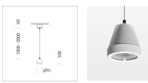
Suspended luminaire with LED, rated life of the LED L80/B10 > 50000 h, chromaticity tolerance 2 SDCM (initial), reflector with circular light distribution pattern, reflector pure aluminium 99,99% in MIRO-Silver®,segmented and faceted, 3D lens silicon to reduce the proportion of scattered light, luminaire head die-cast aluminium, powder-coated, stratowhite
