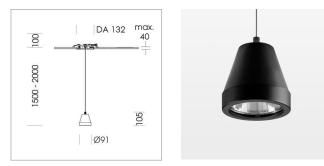
Suspended luminaire with LED, rated life of the LED L80/B10 > 50000 h, colour rendering index CRI > 80, chromaticity tolerance 3 SDCM (initial), rotation-symmetrical reflector with circular light distribution pattern, reflector pure aluminium 99,99% in MIRO-Silver®,segmented and faceted, 3D lens silicon to reduce the proportion of scattered light, luminaire head die-cast aluminium, powder-coated, stratoblack, separate driver unit
