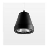
Suspended luminaire with LED, rated life of the LED L80/B10 > 50000 h, colour rendering index CRI > 96, chromaticity tolerance 2 SDCM (initial), rotation-symmetrical reflector with circular light distribution pattern, reflector pure aluminium 99,99% in MIRO-Silver®, segmented and faceted, 3D lens silicon to reduce the proportion of scattered light, luminaire head die-cast aluminium, powder-coated, stratoblack, separate driver unit
