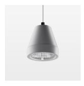
Suspended luminaire with LED, rated life of the LED L80/B10 > 50000 h, colour rendering index CRI > 96, chromaticity tolerance 2 SDCM (initial), rotation-symmetrical reflector with circular light distribution pattern, reflector pure aluminium 99,99% in MIRO-Silver®, segmented and faceted, 3D lens silicon to reduce the proportion of scattered light, luminaire head die-cast aluminium, powder-coated, stratosilver, separate driver unit
