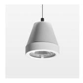
Suspended luminaire with LED, rated life of the LED L80/B10 > 50000 h, colour rendering index CRI > 80, chromaticity tolerance 3 SDCM (initial), rotation-symmetrical reflector with circular light distribution pattern, reflector pure aluminium 99,99% in MIRO-Silver®, segmented and faceted, 3D lens silicon to reduce the proportion of scattered light, luminaire head die-cast aluminium, powder-coated, stratowhite, separate driver unit
