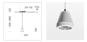
Suspended luminaire with LED, rated life of the LED L80/B10 > 50000 h, colour rendering index CRI > 90, chromaticity tolerance 3 SDCM (initial), rotation-symmetrical reflector with circular light distribution pattern, reflector pure aluminium 99,99% in MIRO-Silver®,segmented and faceted, 3D lens silicon to reduce the proportion of scattered light, luminaire head die-cast aluminium, powder-coated, stratowhite, separate driver unit
