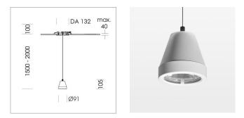
Suspended luminaire with LED, rated life of the LED L80/B10 > 50000 h, colour rendering index CRI > 95, chromaticity tolerance 2 SDCM (initial), rotation-symmetrical reflector with circular light distribution pattern, reflector pure aluminium 99,99% in MIRO-Silver®,segmented and faceted, 3D lens silicon to reduce the proportion of scattered light, luminaire head die-cast aluminium, powder-coated, stratowhite, separate driver unit
