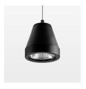
Suspended luminaire with LED, rated life of the LED L80/B10 > 50000 h, colour rendering index CRI > 90, chromaticity tolerance 2 SDCM (initial), rotation-symmetrical reflector with circular light distribution pattern, reflector pure aluminium 99,99% in MIRO-Silver®, segmented and faceted, 3D lens silicon to reduce the proportion of scattered light, luminaire head die-cast aluminium, powder-coated, stratoblack, separate driver unit
