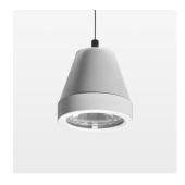
Suspended luminaire with LED, rated life of the LED L80/B10 > 50000 h, colour rendering index CRI > 90, chromaticity tolerance 2 SDCM (initial), rotation-symmetrical reflector with circular light distribution pattern, reflector pure aluminium 99,99% in MIRO-Silver®, segmented and faceted, 3D lens silicon to reduce the proportion of scattered light, luminaire head die-cast aluminium, powder-coated, stratowhite, separate driver unit
