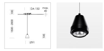
Suspended luminaire with LED, rated life of the LED L80/B10 > 50000 h, colour rendering index CRI > 80, chromaticity tolerance 2 SDCM (initial), reflector with circular light distribution pattern, reflector pure aluminium 99,99% in MIRO-Silver®,segmented and faceted, 3D lens silicon to reduce the proportion of scattered light, luminaire head die-cast aluminium, powdercoated, stratoblack, separate driver unit
