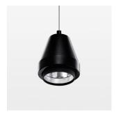
Suspended luminaire with LED, rated life of the LED L80/B10 > 50000 h, colour rendering index CRI > 90, chromaticity tolerance 2 SDCM (initial), reflector with circular light distribution pattern, reflector pure aluminium 99,99% in MIRO-Silver®, segmented and faceted, 3D lens silicon to reduce the proportion of scattered light, luminaire head die-cast aluminium, powder-coated, stratoblack, separate driver unit
