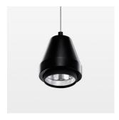
Suspended luminaire with LED, rated life of the LED L80/B10 > 50000 h, colour rendering index CRI > 96, chromaticity tolerance 3 SDCM (initial), reflector with circular light distribution pattern, reflector pure aluminium 99,99% in MIRO-Silver®, segmented and faceted, 3D lens silicon to reduce the proportion of scattered light, luminaire head die-cast aluminium, powder-coated, stratoblack, separate driver unit
