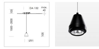
Suspended luminaire with LED, rated life of the LED L80/B10 > 50000 h, colour rendering index CRI > 90, chromaticity tolerance 2 SDCM (initial), reflector with circular light distribution pattern, reflector pure aluminium 99,99% in MIRO-Silver®,segmented and faceted, 3D lens silicon to reduce the proportion of scattered light, luminaire head die-cast aluminium, powdercoated, stratoblack, separate driver unit
