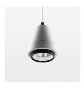
Suspended luminaire with LED, rated life of the LED L80/B10 > 50000 h, colour rendering index CRI > 80, chromaticity tolerance 2 SDCM (initial), reflector with circular light distribution pattern, reflector pure aluminium 99,99% in MIRO-Silver®, segmented and faceted, 3D lens silicon to reduce the proportion of scattered light, luminaire head die-cast aluminium, powder-coated, stratowhite, separate driver unit
