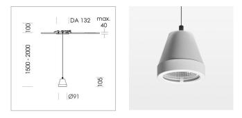
Suspended luminaire with LED, rated life of the LED L80/B10 > 50000 h, colour rendering index CRI > 80, chromaticity tolerance 2 SDCM (initial), reflector with circular light distribution pattern, reflector pure aluminium 99,99% in MIRO-Silver®,segmented and faceted, 3D lens silicon to reduce the proportion of scattered light, luminaire head die-cast aluminium, powdercoated, stratowhite, separate driver unit
