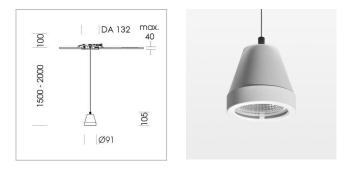
Suspended luminaire with LED, rated life of the LED L80/B10 > 50000 h, colour rendering index CRI > 90, chromaticity tolerance 2 SDCM (initial), reflector with circular light distribution pattern, reflector pure aluminium 99,99% in MIRO-Silver®,segmented and faceted, 3D lens silicon to reduce the proportion of scattered light, luminaire head die-cast aluminium, powdercoated, stratowhite, separate driver unit
