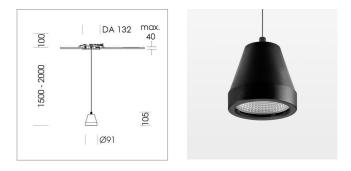
Suspended luminaire with LED, rated life of the LED L80/B10 > 50000 h, colour rendering index CRI > 80, chromaticity tolerance 2 SDCM (initial), reflector with circular light distribution pattern, reflector pure aluminium 99,99% in MIRO-Silver®,segmented and faceted, luminaire head die-cast aluminium, powder-coated, stratoblack, separate driver unit
