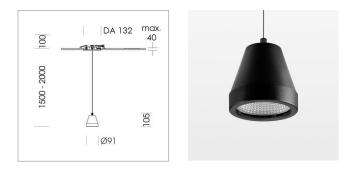
Suspended luminaire with LED, rated life of the LED L80/B10 > 50000 h, colour rendering index CRI > 90, chromaticity tolerance 2 SDCM (initial), reflector with circular light distribution pattern, reflector pure aluminium 99,99% in MIRO-Silver®,segmented and faceted, luminaire head die-cast aluminium, powder-coated, stratoblack, separate driver unit
