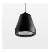
Suspended luminaire with LED, rated life of the LED L80/B10 > 50000 h, chromaticity tolerance 2 SDCM (initial), reflector with circular light distribution pattern, reflector pure aluminium 99,99% in MIRO-Silver®, segmented and faceted, luminaire head die-cast aluminium, powdercoated, stratoblack, separate driver unit
