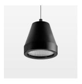
Suspended luminaire with LED, rated life of the LED L80/B10 > 50000 h, colour rendering index CRI > 96, chromaticity tolerance 3 SDCM (initial), reflector with circular light distribution pattern, reflector pure aluminium 99,99% in MIRO-Silver®, segmented and faceted, luminaire head die-cast aluminium, powder-coated, stratoblack, separate driver unit
