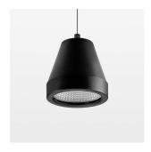
Suspended luminaire with LED, rated life of the LED L80/B10 > 50000 h, colour rendering index CRI > 90, chromaticity tolerance 2 SDCM (initial), reflector with circular light distribution pattern, reflector pure aluminium 99,99% in MIRO-Silver®, segmented and faceted, luminaire head die-cast aluminium, powder-coated, stratoblack, separate driver unit
