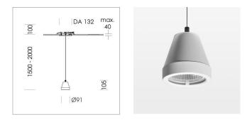
Suspended luminaire with LED, rated life of the LED L80/B10 > 50000 h, colour rendering index CRI > 96, chromaticity tolerance 3 SDCM (initial), reflector with circular light distribution pattern, reflector pure aluminium 99,99% in MIRO-Silver®,segmented and faceted, luminaire head die-cast aluminium, powder-coated, stratowhite, separate driver unit
