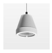
Suspended luminaire with LED, rated life of the LED L80/B10 > 50000 h, colour rendering index CRI > 90, chromaticity tolerance 2 SDCM (initial), reflector with circular light distribution pattern, reflector pure aluminium 99,99% in MIRO-Silver®, segmented and faceted, luminaire head die-cast aluminium, powder-coated, stratowhite, separate driver unit
