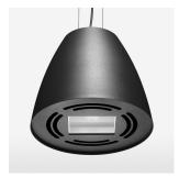
Suspended luminaire with LED, rated life of the LED L80/B10 > 50000 h, colour rendering index CRI > 90, chromaticity tolerance 2 SDCM (initial), reflector with double asymmetrical light distribution pattern, reflector pure aluminium 99,99% in MIRO-Silver®, luminaire housing sheet steel, powdercoated, stratoblack
