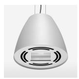
Suspended luminaire with LED, rated life of the LED L80/B10 > 50000 h, colour rendering index CRI > 90, chromaticity tolerance 2 SDCM (initial), reflector with double asymmetrical light distribution pattern, reflector pure aluminium 99,99% in MIRO-Silver®, luminaire housing sheet steel, powdercoated, stratowhite
