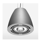
Suspended luminaire with LED, rated life of the LED L80/B10 > 50000 h, colour rendering index CRI > 80, chromaticity tolerance 2 SDCM (initial), reflector with circular light distribution pattern, reflector pure aluminium 99,99% in MIRO-Silver®, swivel angle 2x25°, luminaire housing sheet steel, powder-coated, stratosilver
