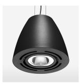
Suspended luminaire with LED, rated life of the LED L80/B10 > 50000 h, colour rendering index CRI > 80, chromaticity tolerance 2 SDCM (initial), reflector with circular light distribution pattern, reflector pure aluminium 99,99% in MIRO-Silver®, swivel angle 2x25°, luminaire housing sheet steel, powder-coated, stratoblack
